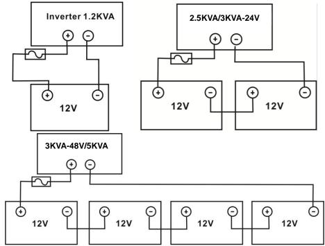
4. For 1.2KVA/2.5KVA/3KVA-48V/5KVA models, insert the battery wires flatly into battery connectors of inverter and make sure the bolts are tightened with torque of 2 Nm in clockwise direction. Make sure polarity at both the battery and the inverter/charge is correctly connected and conductors are tightly screwed into the battery terminals.
