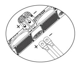
5. This step is only for 1.2KA/2.5KVA/3KVA-48V/5KVA models. To firmly secure wire connection, you may fix the wires to strain relief with cable tie.
