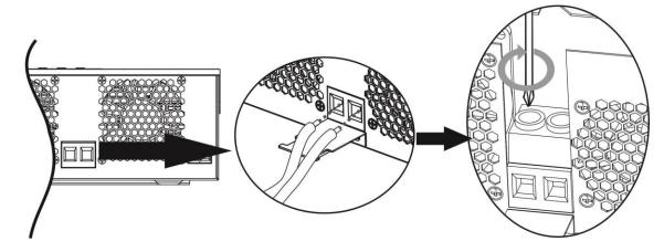
For 3K-24V model, secure assembled ring terminals to the battery terminal block with the bolts properly tightened. Refer to battery cable size for torque value. Make sure polarity at both the battery and the inverter is correctly connected and ring terminals are secured to the battery terminals.
