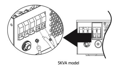
5. Make sure the wires are securely connected.
